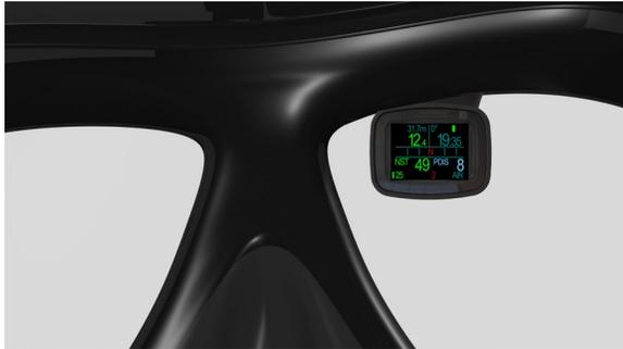
their dive data without losing eye contact with their surroundings, or having to constantly refocus. Dive information is displayed on the micro OLED screen protected in the housing, offering durability and superior readability in any ambient light conditions.
